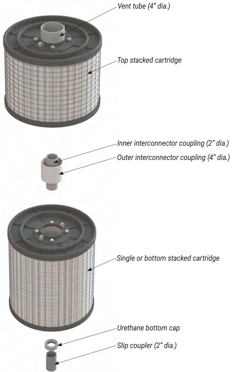
**Figure 3. Schematic of stacked cartridges and connector components.**
