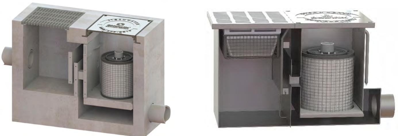
These systems have a maximum depth of 5 feet from the rim to the invert of the outlet pipe. The minimum depth is dictated by the cartridge stack height. The catch basin configuration can also accommodate an inlet pipe if needed, and includes a high-flow bypass that routes peak flows around the treatment chamber to discharge.
