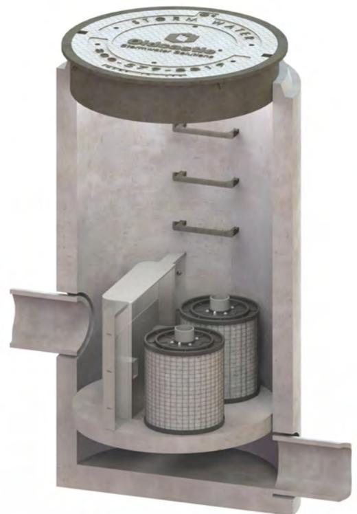
**Vault:** The standard Vault PerkFilter can contain up to 31 cartridge stacks and is provided in a precast concrete vault ranging in size from 4' x 4' up to 8' x 18'. Stormwater is typically delivered to the Vault PerkFilter through an inlet pipe connection. The Vault PerkFilter includes a high-flow bypass that routes peak flows around the treatment chamber to discharge.
